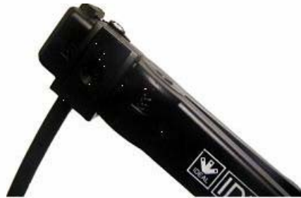
2. Place cable in stripper with 1/4" protruding
