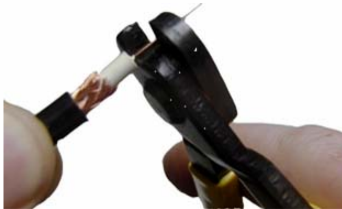
2. Lay side of cutter against white dielectric, ensure center conductor length is 0.187" (about 4.8mm)
