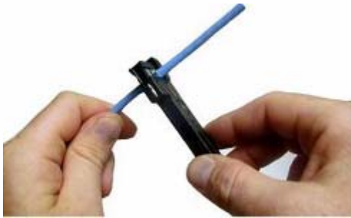
Ring cable about 3" from end to score sheathing
