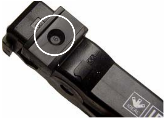
1. Set sliding window to cable size
