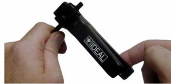
3. Rotate stripper in direction of lettering
