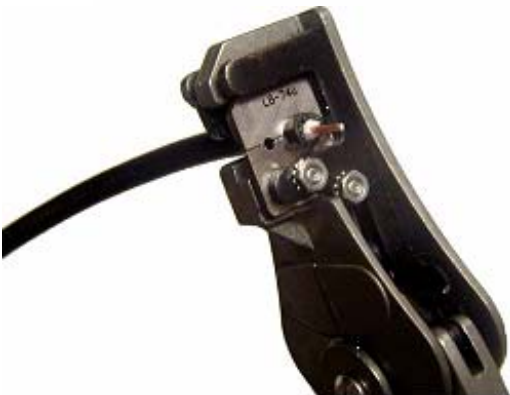
3. Place cable in larger hole 1/4" protruding, squeeze
