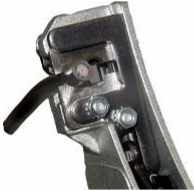
1. Place cable in smaller hole 1/2" protruding
