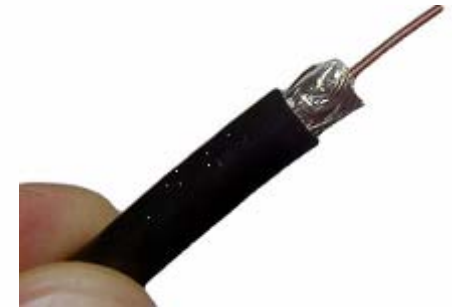
6. Stripped cable for F-style
