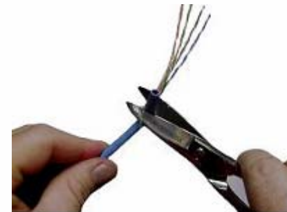
Cut away excess sheathing and ripcord
